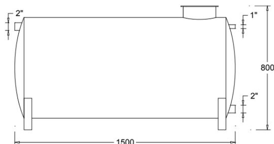
Priming tank 500 liter, galvanized steel complete with:
